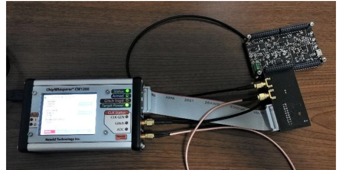
8. Figure 8 Picture of a RAMN board connected to ChipWhisperer Pro through a dedicated expansion board.
