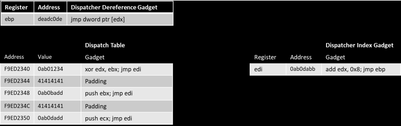
Figure 9. Two-gadget dispatcher, utilizing a jmp in the dispatcher index gadget.
